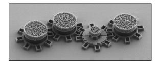
Researchers at the University of Gothenburg have developed the world's smallest light-powered gears, microscopic machines so tiny they can fit inside a single strand of hair. Each gear, only about 0.016 millimeters in diameter, is made of silica and features an optical metamaterial that reacts to laser light, allowing it to move without any mechanical contact.
