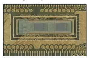
The optical chip integrates lasers and microscopic Fresnel lenses, thinner than a human hair, onto a circuit board. Data from images or other inputs are converted into laser light, processed through these lenses, and then reconverted into digital signals, completing AI computations with minimal energy use and faster speeds.
